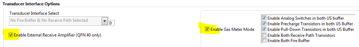
Figure 11: Setting gas meter mode in GUI
