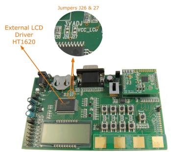
The following picture shows the connection of an external LCD driver circuit:
