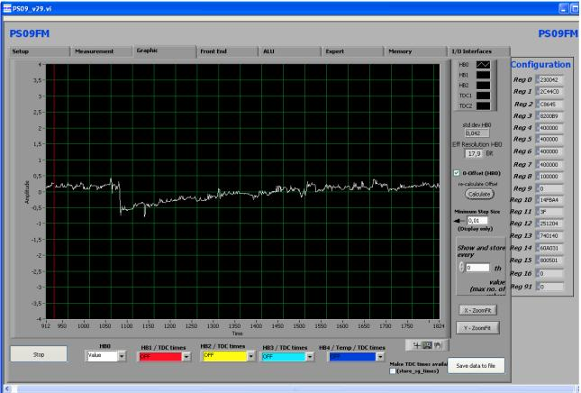
Graphical display of the results. The consolidated result HBO as well as the separate half bridge results can be displayed. Additionally, Temperature can also be graphically displayed.
