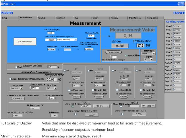
Measurement valueDisplay of HBO result using the software filters set under "Filter".Eff. ResolutionEffective resolution with respect to maximum outputFilterSelection of various software filters like SINC (rolling average) and Median (non-linear filter).
