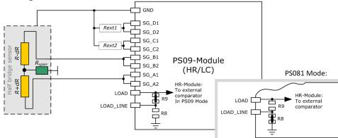
An alternative way of connecting a half bridge to PSØ9 is shown below, where the unused ports C and D are connected parallel to Ports A and B respectively. The external resistors are avoided in this connection. The option for using an external comparator is available only on the HR-module.
