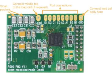
Figure 2-1: High Resolution Module
