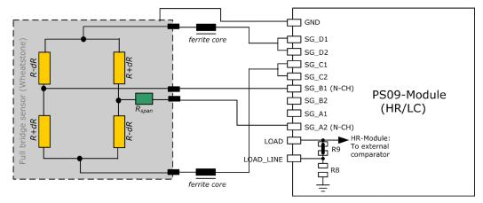
The PICOSTRAIN measurement principle is based on measuring the discharge time of a capacitor. For this reason the correct size and material of the capacitors is significant to achieve best measuring results. For Wheatstone, the discharging time is furthermore reduced by the factor of 0.7, The following formula can be used to calculate the discharging capacitance.
