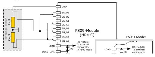
Please note: Both wiring options shown in figure 3a and 3b have to be done externally, i.e. at the solder pad of the module. There are no wiring or placement options on the module itself.
