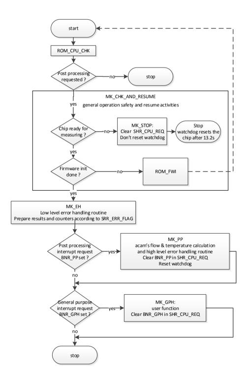
The routine **MK\_PP** is the major calculation and high level error handling routine. Its internal structure is sketched below.
