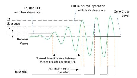
The essential difference of this method compared to methods 1 and 2 is that the active FHL can be arbitrarily different from the trusted FHL. For example, the trusted FHL may be suitable for detecting the second wave as first hit, over all temperatures and tolerances. But it may feature low EMI clearance (small differences between neighboring wave amplitudes), such that a later wave with higher amplitude and higher clearance may be preferable, for example the fourth wave. Now the
