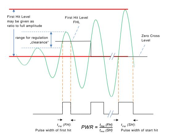
This is the first important step of the FHL selection. Until here, it is not related to acam firmware and can be used in remote control operation as well. But now it should be noted that the result of the selection process described above can change over temperature, production tolerances and aging; for some devices and transducers it may even depend on flow and pressure. The problem is to
