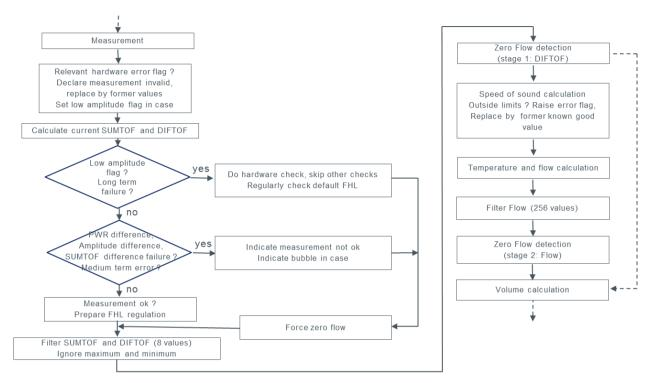
A number of decisions depends strongly on the frequency of events and the duration of errors. Information on error counts can be retrieved from the error counters described in the next section. The following numbers are important for error handling and flow calculation as well as for first hit level regulation and zero flow detection:
