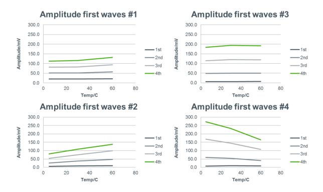
These example plots demonstrate how different receive wave amplitudes - and with them the corresponding FHL levels – can vary over temperature for different spool pieces #1 - #4. Accordingly, different spool pieces require different FHL regulation methods for stable first hit detection.
